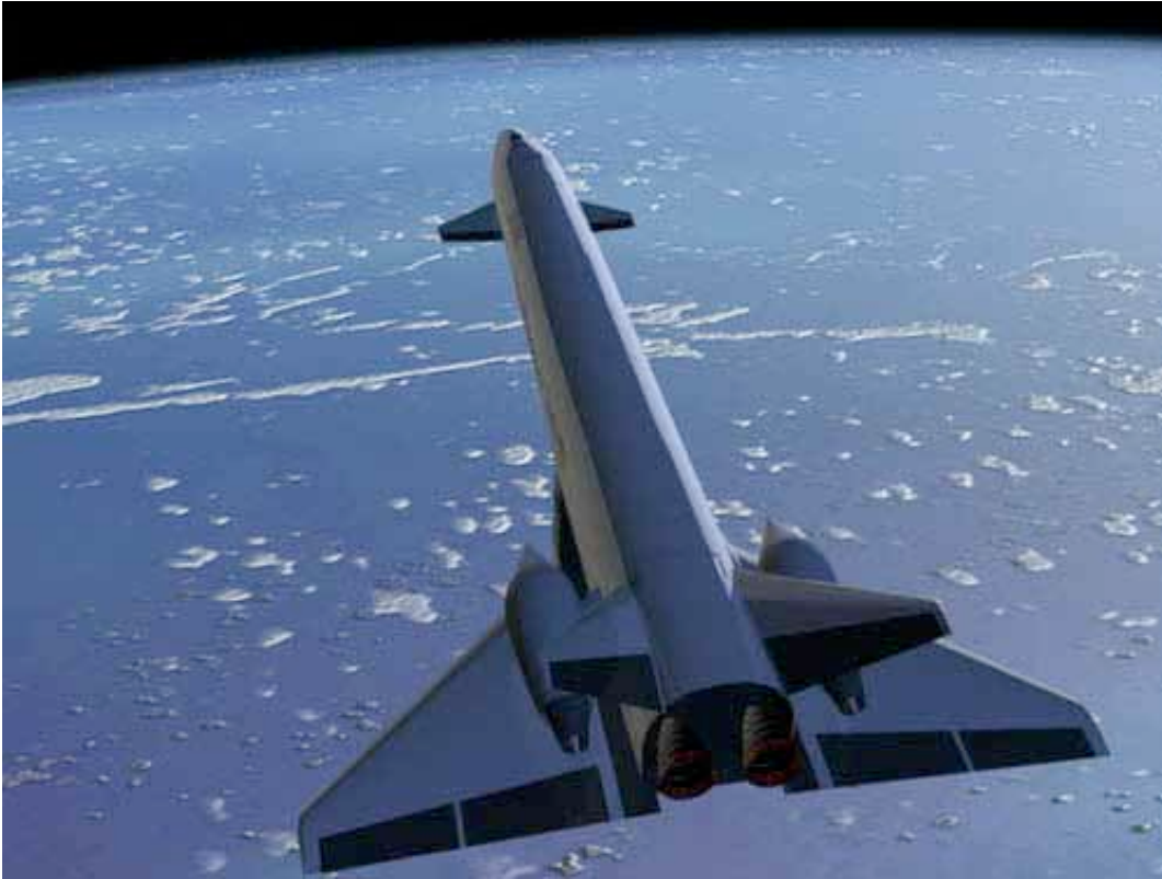
StarBooster 200 on its return flight after lifting an upper-stage to the outer reaches of the atmosphere
