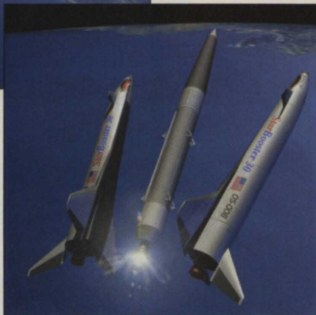
Starcraft has designed a fly-back-booster-based launch system to reduce costs.
